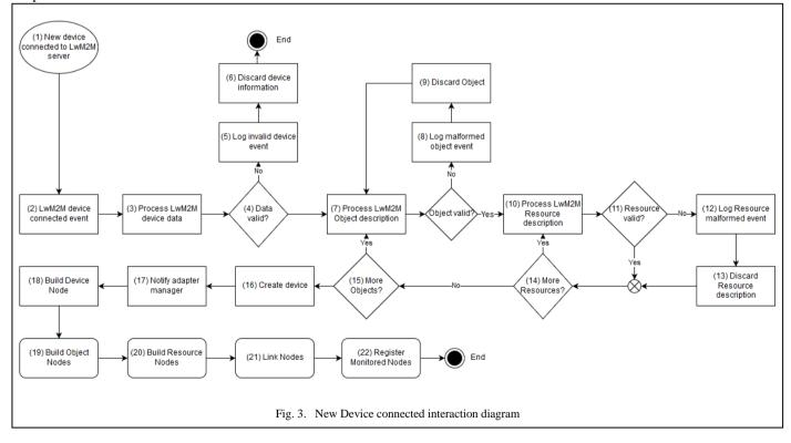
Typically, *Resource Nodes* (20) are the only *Node* types that have real data. However as described in the following section, we allow specific *Object Nodes* (19) to contain it as well. This property is identified by the IPSO description, and specifies whether the *Node* can be monitored for value changes. Once all of the *Children Nodes* are linked (21) to the *Device Node*, the system checks, which of *Nodes* have the *Observable* property and be registers them for monitoring (22).
