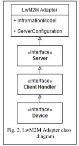
outgoing LwM2M events and commands. *Server interface* internally depends on the *Client Handler interface* that handles various LwM2M events generated by the LwM2M Client, and keeps track of all know LwM2M Device within the network.
